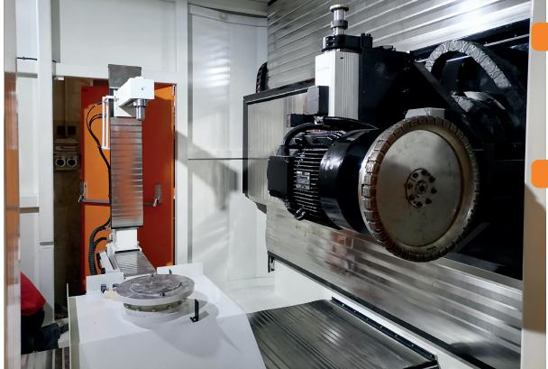
Because of the special triple design of Diamond grinds; the grinding, cutting, hole grinding can be done without changing grinds.
